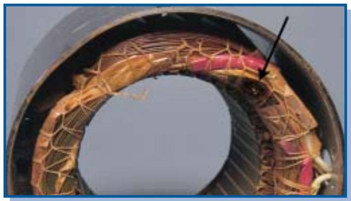
This winding fault was caused by a voltage surge. An insulation test will not detect it!
